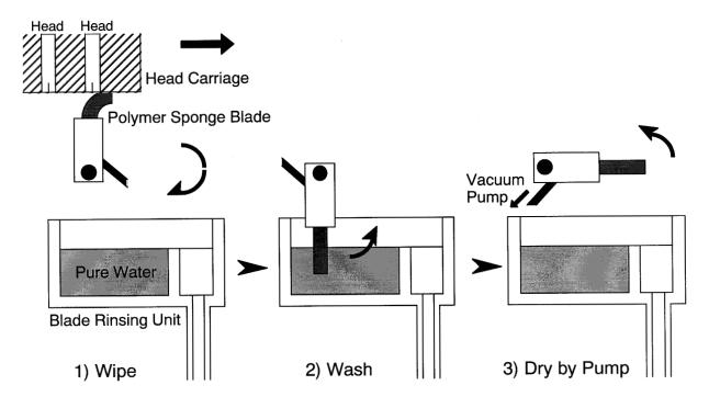
Figure 6. Process flow of the New Head Cleaning System
