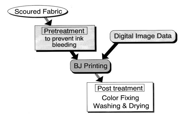
Figure 2. Process flow of the system
